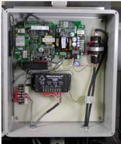
Optional integrated enclosure with base station, Smart Node, interrupter and 100A Hg mercury relay
