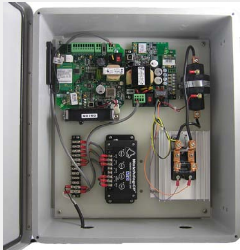
Base unit in enclosure with Smart Node, interrupter and solid state relay options
